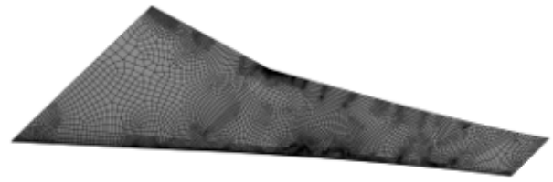
Figure 2: Converged mesh of wing structure
