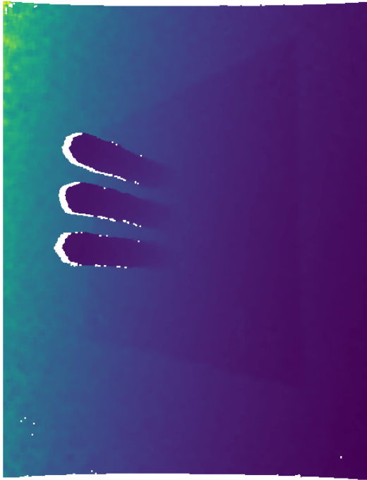
Figure F.7. Initial depth map captured by the iPhone (insufficient quality).
