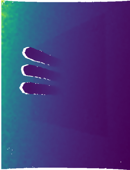
Figure 14. Initial depth map captured by the iPhone (insufficient quality).
