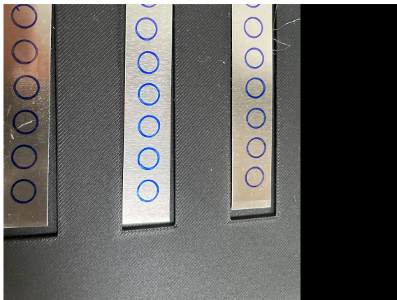
Figure 2. Tantalum-sputtered aluminum slides with micro-patterned antigen wells.
